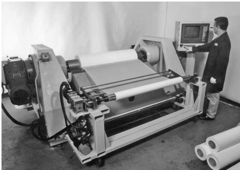
FIGURE 4.8 Modern skiving machine. (Courtesy of Dalau Inc.)
