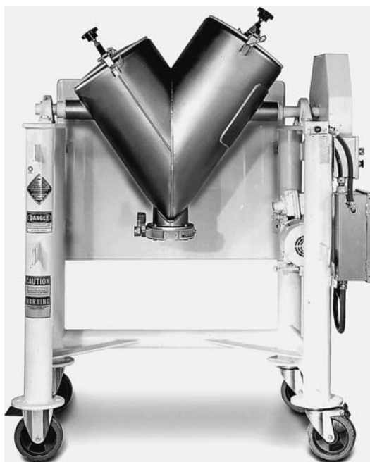
FIGURE 4.10 Twin shell blender. (Courtesy of Patterson-Kelley Co.)
