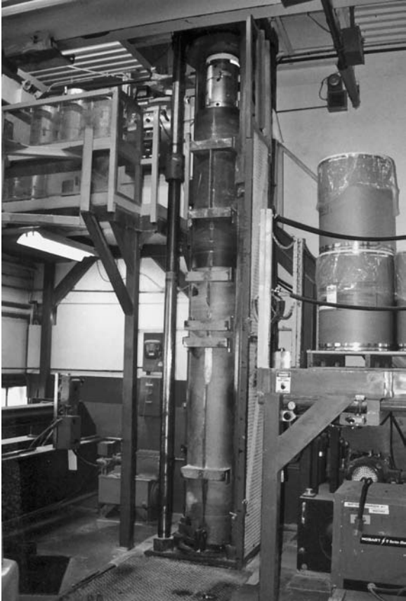
FIGURE 4.2 Compression molding press for PTFE billets.
